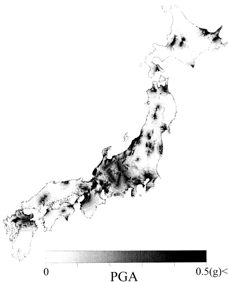
図2 今後50年間に10%の確率で被ると予想される地震動（最大加速度）マップ Figure 2 Map of horizontal peak ground acceleration (PGA) expected at 10% or higher probability for next 50 years, under Poisson earthquake occurrence hypothesis. The attenuation relation used is the equation of Fukushima and Tanaka (1990), based on surface geology.
