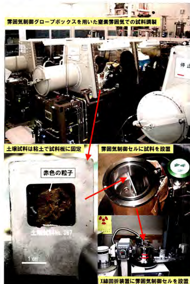
図6 窒素雰囲気における腐食生成物の試料調製方法 Fig. 6 Sample preparation for X-ray diffraction analysis of copper corrosion products under a protective nitrogen atmosphere
