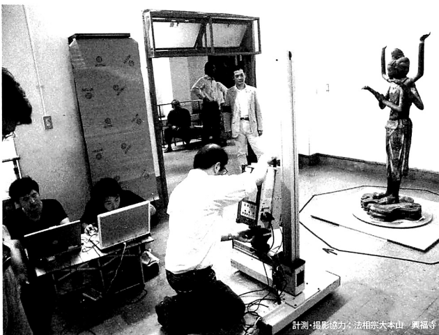
図6 阿修羅像の三次元計測風景 Fig. 6 Making a 3D measurement of Asura statue (national treasure) belonging to Kofukuji Temple
