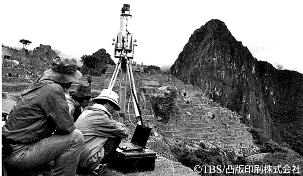
図8 マチュ・ピチュ遺跡の三次元計測風景 Fig. 8 Making a 3D measurement of the historic sanctuary of Machu Picchu (UNESCO world heritage site)
