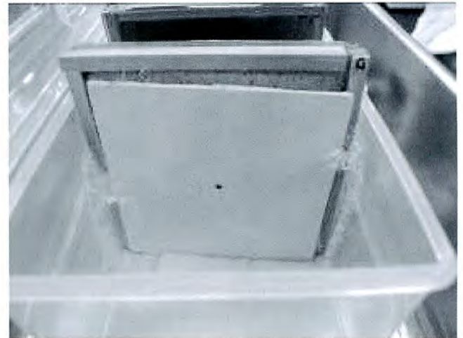
図 17 劣化促進実験終了後の試験片 B Fig. 17 Appearance of test piece B after the accelerated ageing experiment ; the plaster layer was completely exfoliated from the sand plaster layer
