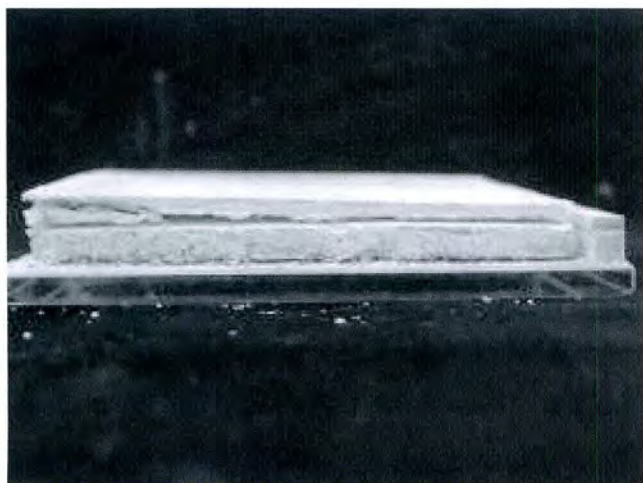
図 20 側面から見た劣化促進実験後の試験片 B の断面；試験片下部 (写真の左側) の漆喰層は膨張し、上部 (右側) は変化がない Fig. 20 Cross section of test piece B after the accelerated ageing experiment observed from its side, showing exfoliated plaster layers of the lower part (left side in photo) and unchanged the upper part (right side)
