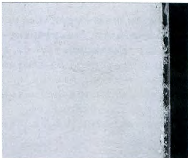
図 21 劣化促進実験後の試験片 B の砂漆喰層表面 Fig. 21 Surface appearance of the sand plaster layer of test piece B after the accelerated ageing experiment
