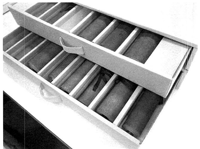
写真7 中性紙で作製した保存箱 Photo 7 Preservation box that was made by neutral paper.
