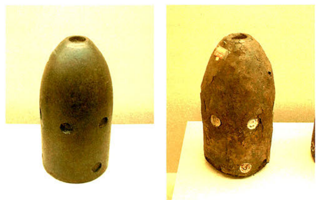
図1 脱塩の効果（左：処理済、右：未脱塩） Fig. 1 Impact of desalination (Left: treated, Right: untreated)
