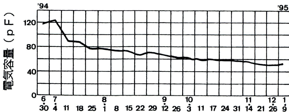
図5 コンクリート屋根スラブ内水分挙動に伴う電気容量の経時変化 Fig. 5 The hourly variation of electric capacity accompanied with moisture behavior in a concrete roof structure
