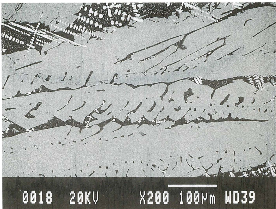
写真2 山田地蔵谷 (YMJ-03) 出土鉄滓 (ファヤライト+酸化鉄) Photo.2 Back scattered electron image of slag at Yamada-Jizodani ruins, YMJ03, (showing fayalite and iron oxide).
